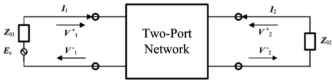
Fig. 3. Schematic diagram of two-port network showing network voltage variables.
